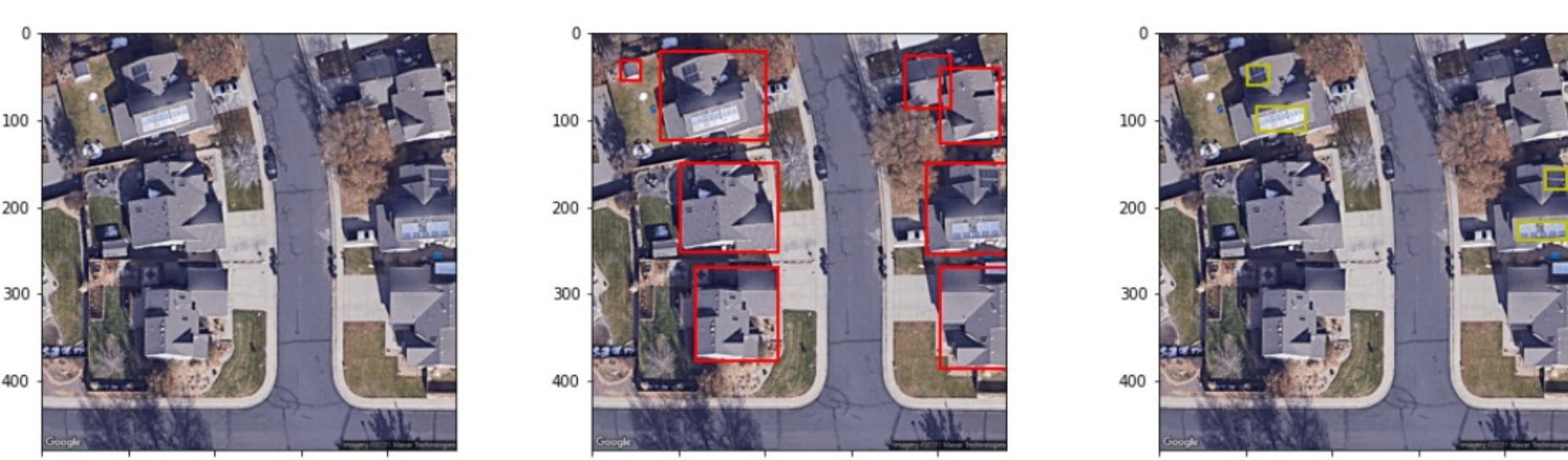
Figure 2. (a) Original (b) Roofs (c) Solar PV
